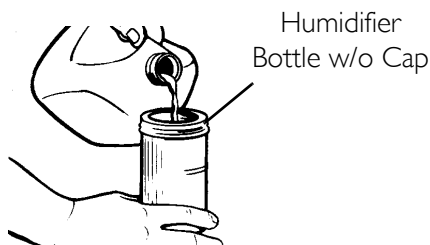
FIGURE 6.1 Filling the Humidifier
